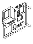
Pin pitch of NCH8200HV is suitable for universal board or breadboard  $% \left( 1\right) =\left( 1\right) \left( 1\right$
